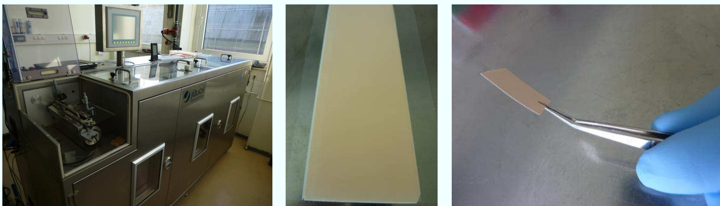
Fig.3: (l.) A tape casting line at IEK-1 can be used for large scale tape casting. (m.) Al-LLZ tapes were successfully processed by tape casting with a gap size of 250 μm and 500 μm. (r.) Solid electrolytes with a green tape thickness of 90 μm and 180 μm were used for further sintering studies.
